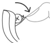
Use the nail grip to gently swing the battery door open and remove the old battery.
